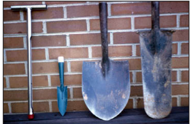
Figure 1. From left to right: a stainless steel soil probe, a hand garden trowel, shovel, and a spade. All acceptable tools for collecting a soil sample.
